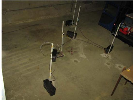
Figure 2: Monitoring system around injection point (red mark in the middle)
