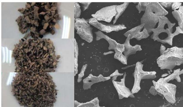
**Figure 1** Left: HAPb fractions, size l: 2-4 mm (top left), m: 0.85-2 mm (middle left) and s: 0.105-0.85 mm (bottom left). Right: SEM image of HAPb particles.
