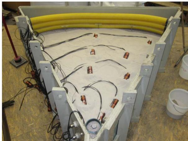
**Figure 3: Large scale container during installation of coils (inflow in front, outflow in the rear)**
