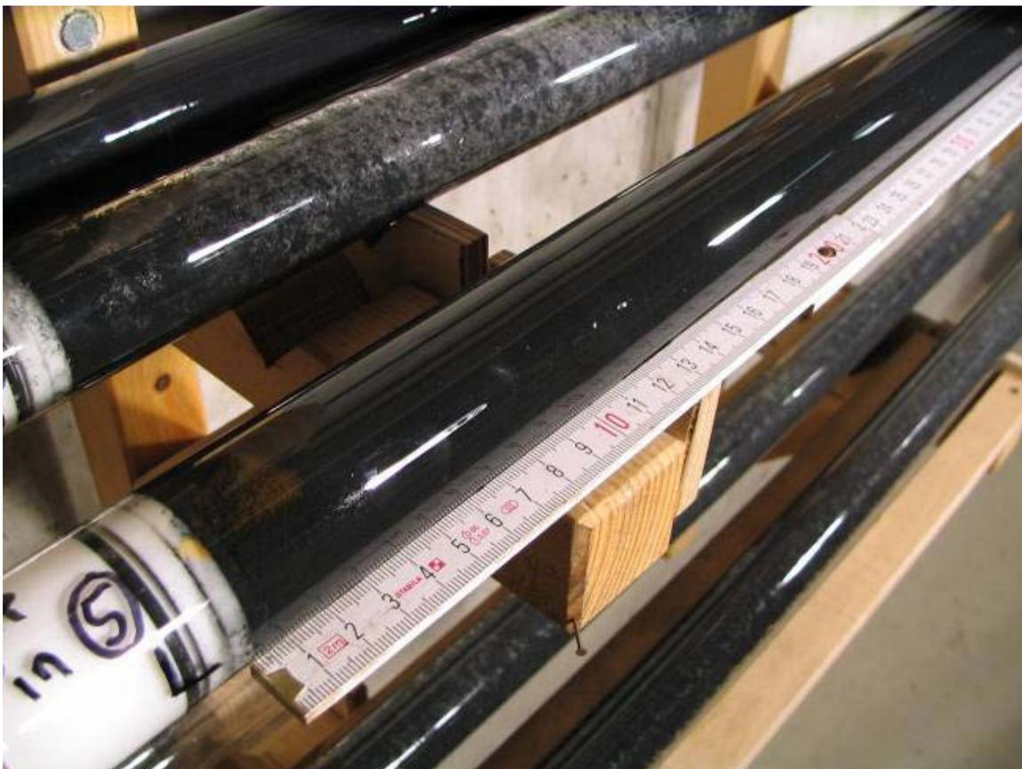
**Figure 2: Columns during longterm experiments. 1 = Reduction of anaerobic corrosion due to addition of  $\text{Ca}(\text{OH})_2$ . 2 = Clogging of the porous media due to the production of hydrogen gas during the anaerobic corrosion (without  $\text{Ca}(\text{OH})_2$ ).**
