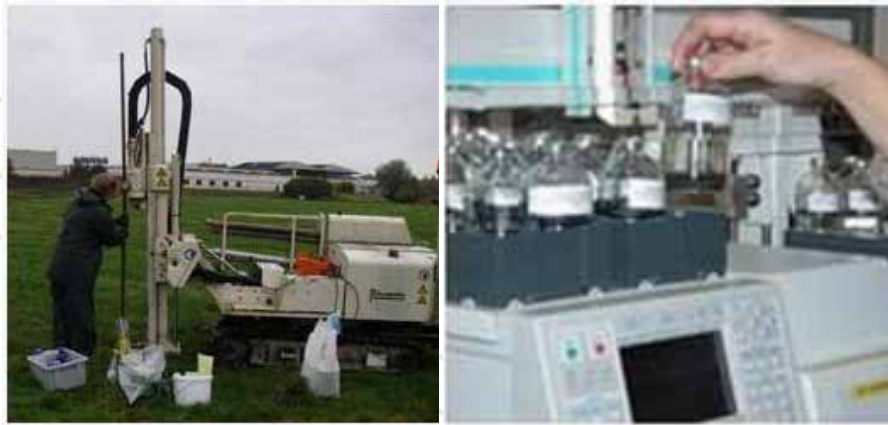
Figure 2: Sampling of undisturbed aquifer and groundwater in the field (Antwerp, Belgium) (left) and laboratory CAH-degradation tests (right)
