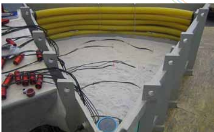
Figure 6: Triangular container for the positioning of sensors in the "field" to detect Fe-based reactive materials
