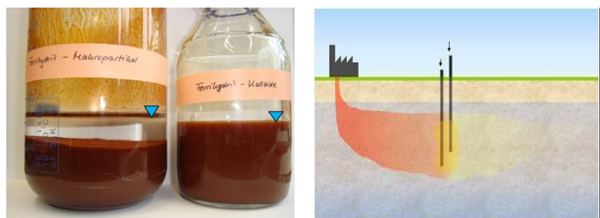
Figure 1: Injectable Fe-oxide particles (left) to create reactive zones for groundwater treatment (right)
