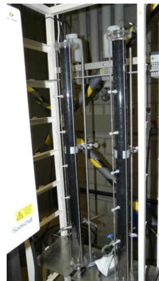
Figure 9 Example of a column test setup with mulch (50 vol%), soil (50 vol%) and groundwater.
