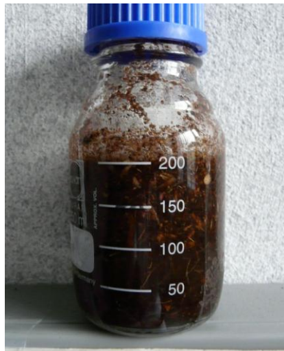
Figure 8 A batch test bottle with mulch, soil and groundwater.
