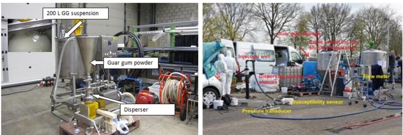
Figure 35 Dispersing unit (Ytron ZC-0) used within AQUAREHAB during pilot test 2 & 3 to prepare 10 m<sup>3</sup> of guar gum suspension in the field.
