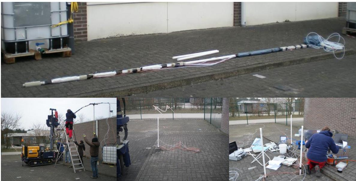
Figure 39. Installation of the multilevel monitoring systems at the Field for a AQUAREHAB pilot test (installation up to 7 m bgs).
