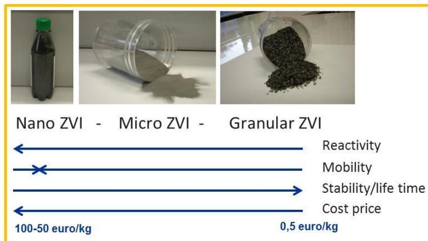
**Figure 3 Comparison of different sized ZVIs.**
