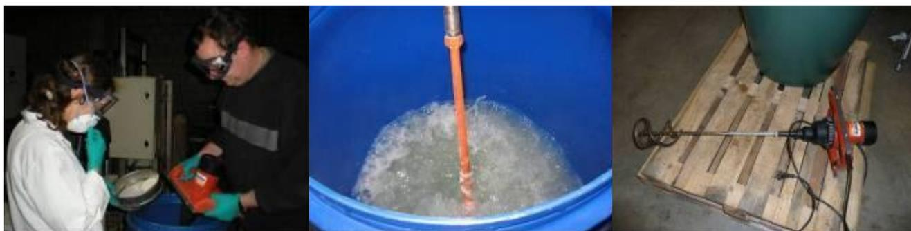
**Figure 33** Guar gum preparation as was performed within SQUAREHAB for a small pilot test (1.6 m<sup>3</sup> ZVI suspension).
