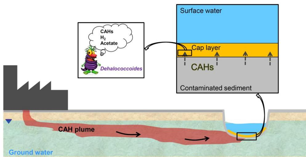
Fig. 1.5. Schematic presentation of the bioreactive cap concept.
