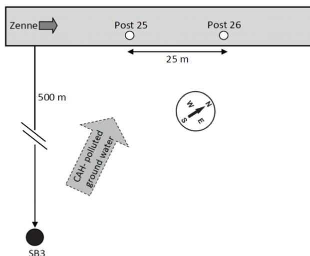
Fig. 2.2. Schematic overview of the test site and locations of post P26, and P25 and the monitoring well SB3.
