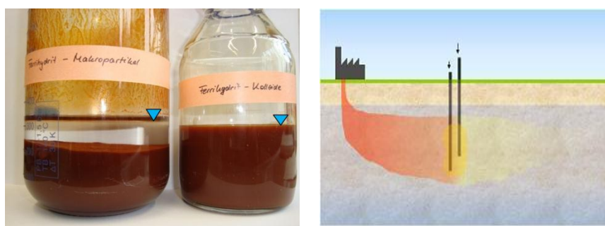
Figure 1: Injectable Fe-based particles (left) to create reactive zones for groundwater treatment (right)
